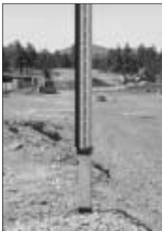
Rod extension fully collapsed
