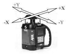
Each end of each axis must be checked for calibration. If needed, the axis can be calibrated using the remote control. You can also take the laser to a service center for calibration.
