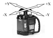
The two horizontal axes (X and Y) are marked near the base of the laser. The ends of the axis are designated as + or - to indicate opposite sides of the axis.
